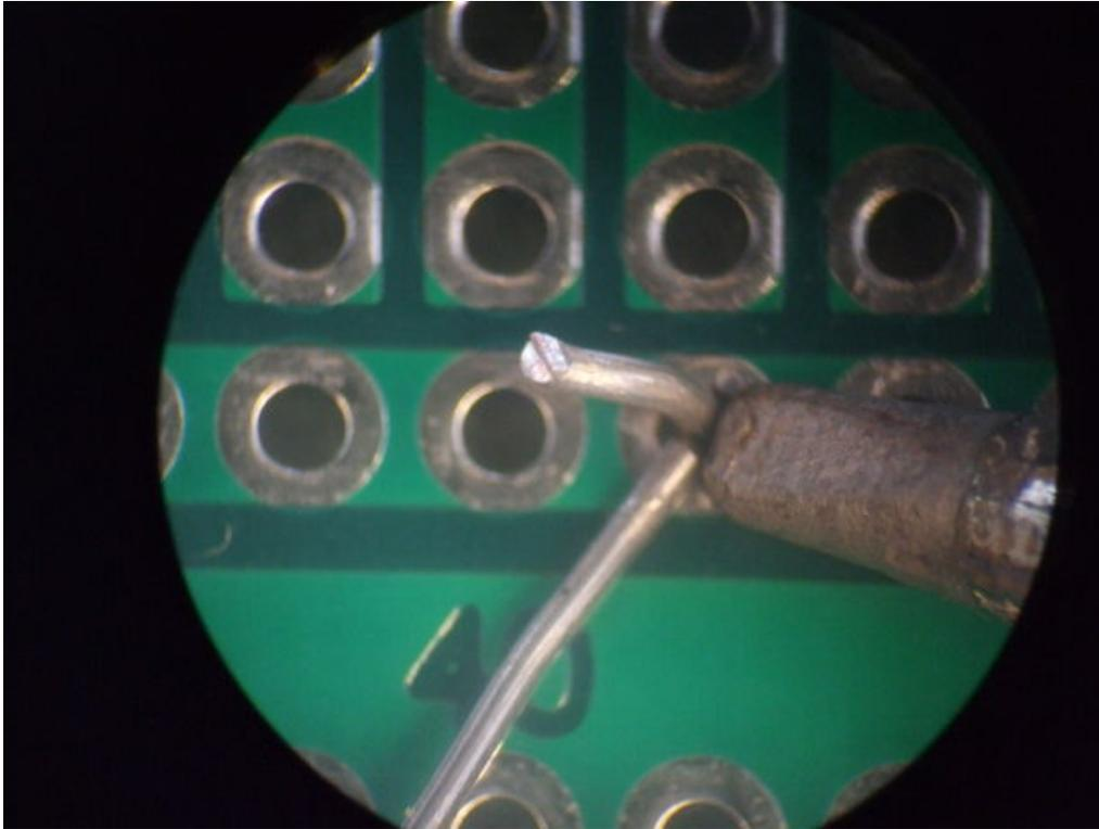
Insert component in circuit board by using a pair of tweezers. If soldering iron is hot enough, take it from stand and hold it as a pen.
