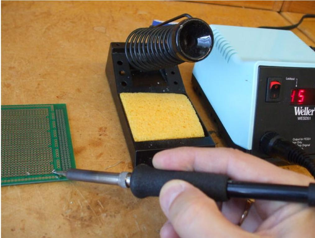
Soldering is process of joining two metals together with soldering iron by the use of a solder to form a dependable electrical joint.
