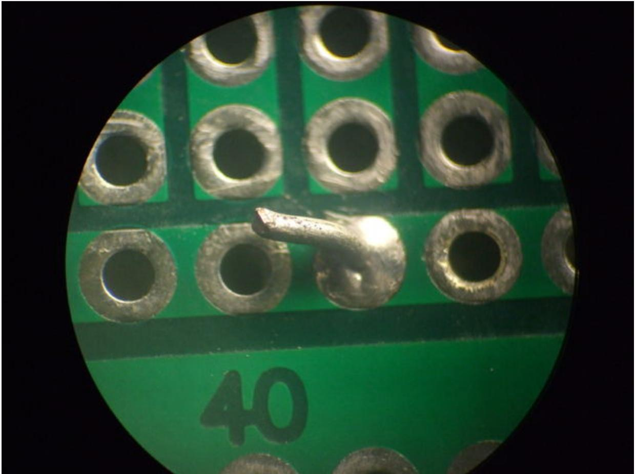
Immediately after soldering, start visual inspection of solder joint. Good magnifying lamp (or a microscope) is required for proper and thorough inspection. Use an ohm-meter to test a solder joint for continuity.
